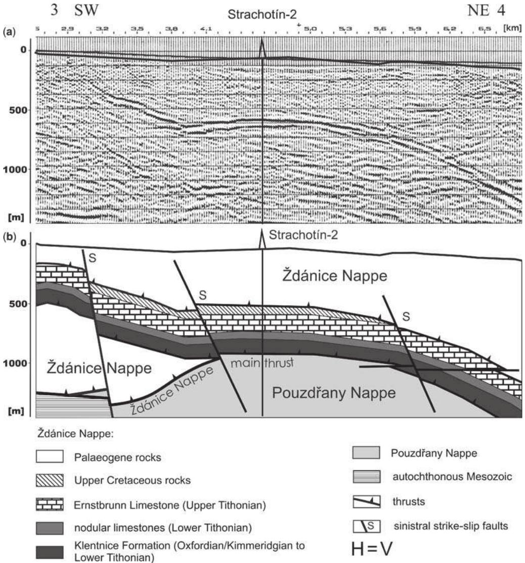
**Fig. 8.** Longitudinal seismic profile 293/83 including a projected borehole (a) and locally balanced cross section (b) obtained from the geological interpretation of the seismic profile shown in (a). See Figure 4 for location of line 3–4.
