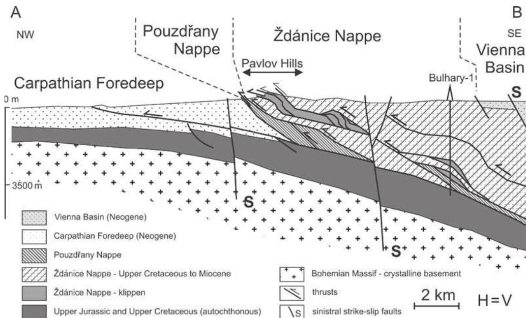
Fig. 2. Conceptual cross section of the frontal part of the Outer Western Carpathians. See Figure 1 for location of the line A–B.
