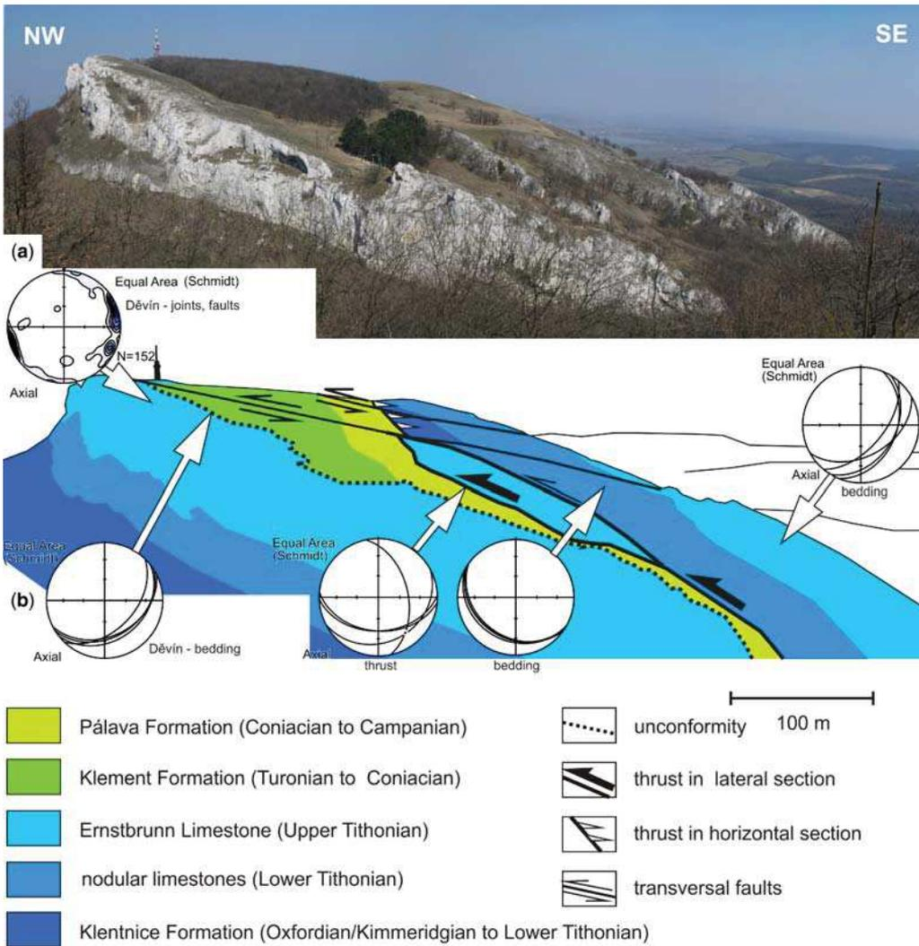
**Fig. 7.** View of SW slope of the Děvín Hill (a) and geological interpretation of the photograph shown in (a) as backlimb of an antiformal structure including a thrust (b). Equal area projections (lower hemisphere) show orientation of structural elements.
