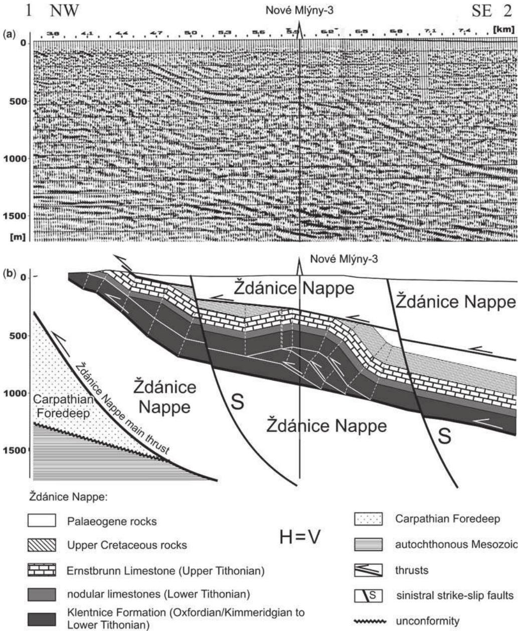
**Fig. 6.** Transversal seismic profile 290/83 including a projected borehole (a) and locally balanced cross section (b) obtained from the geological interpretation of the seismic profile shown in (a). See Figure 4 for location of line 1–2.
