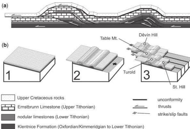
**Fig. 9.** Schematic model of thrust tectonics suitable for the Pavlov Hills (a) and principal stages of its evolution (b). Only Mesozoic rocks are presented, any Tertiary sediments covering this structure are not shown.
